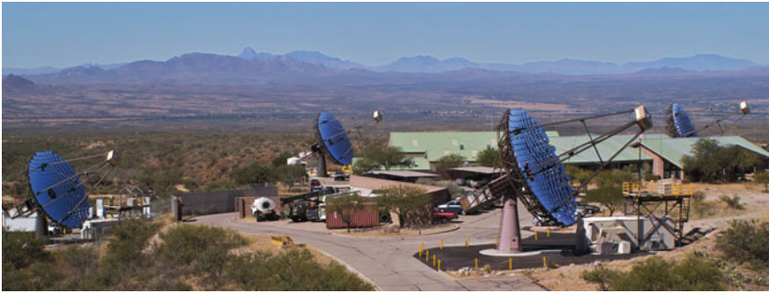
Fig. 28. Photograph of the four VERITAS 12-m diameter Cherenkov telescopes at the Mount Hopkins base camp in Arizona.
