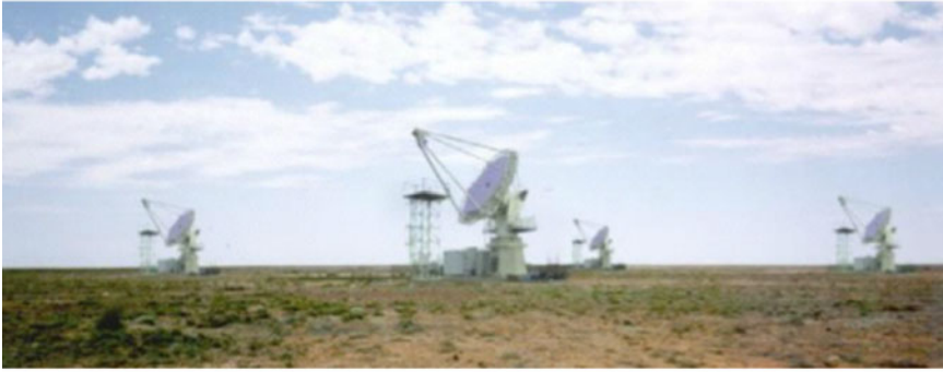
Fig. 24. Photograph of the four Cangaroo III Cherenkov telescopes in the Australian outback. The telescopes were arranged in a diamond pattern. Each telescope had a nearby access tower for servicing the camera. The mirrors had a diameter of 10 m.
